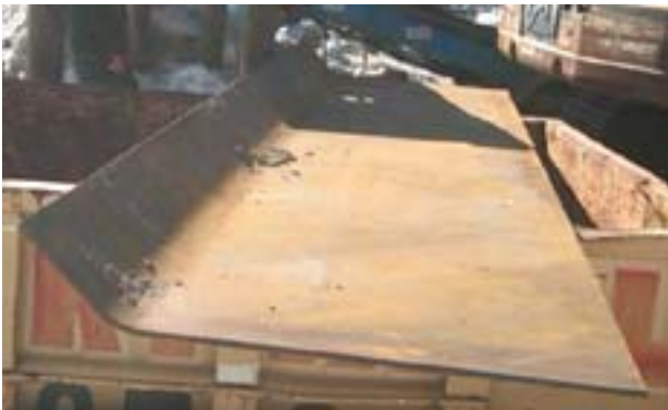
Rock Crusher Hopper Panel STULZ-CREUSABRO 8000
