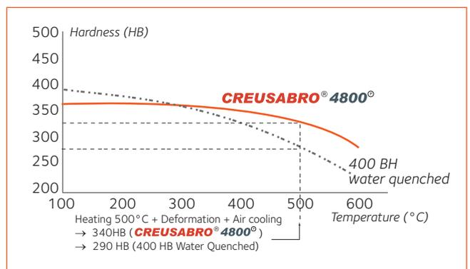
These properties enable the steel to be processed in the hot condition (450/500°C - 840/930°F) : Forming of thick plates, for example, followed by a slow cooling without inducing any significant drop of hardness. Hot resistance of Creusabro® 4800® allows its use in hot environments where pieces are heated up to 350°C (660°F).
