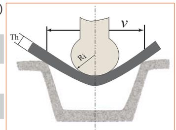
■ The strength necessary to bend depends on UTS and plate thickness as well as bended length and die opening V.
