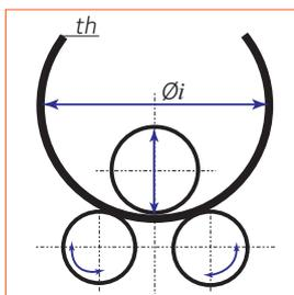
■ Creusabro® 4800® can be hot formed at a temperature of  $450/500^\circ\text{C}$  ( $840/930^\circ\text{F}$ ) without any further heat treatment. At this temperature the force necessary to deform the plate will be lower than at room temperature, and the deformation capability of the steel will be higher (smaller forming radius).
